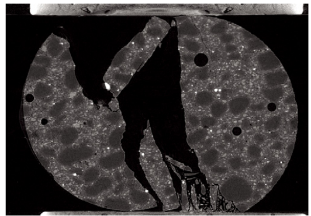
Figure 1: Fractured high strength concrete.
